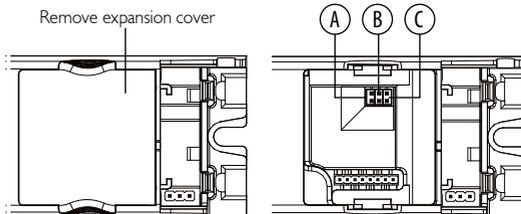
Figure 11: Discharge rating selection
