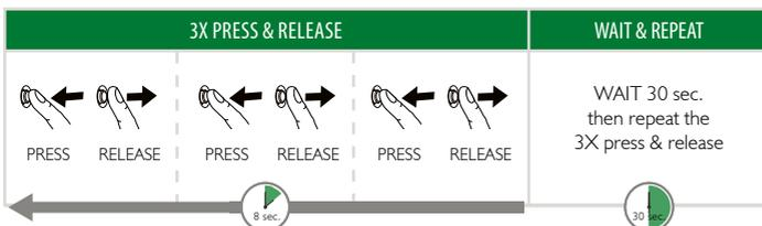
**NOTE:** If the wait in-between breaker or test button push sequences is longer than **50 seconds** then it will timeout and the procedure will need to begin again.
