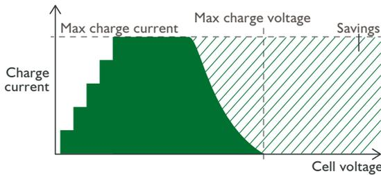
Figure 8: Smart charge rate
