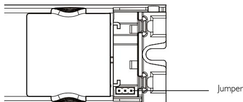
Figure 10: Maintained/non-maintained jumper
