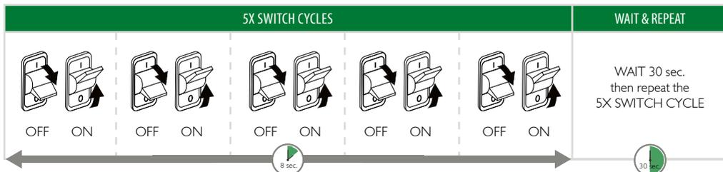
The self test can also be enabled using the test button sequence below:
